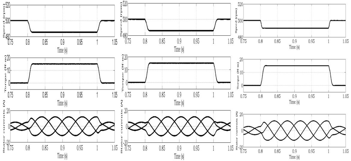
Figure 7. Performance during step change in load torque with Two-level, Three-level and Five- Level inverter fed vector controlled induction motor drive respectively
