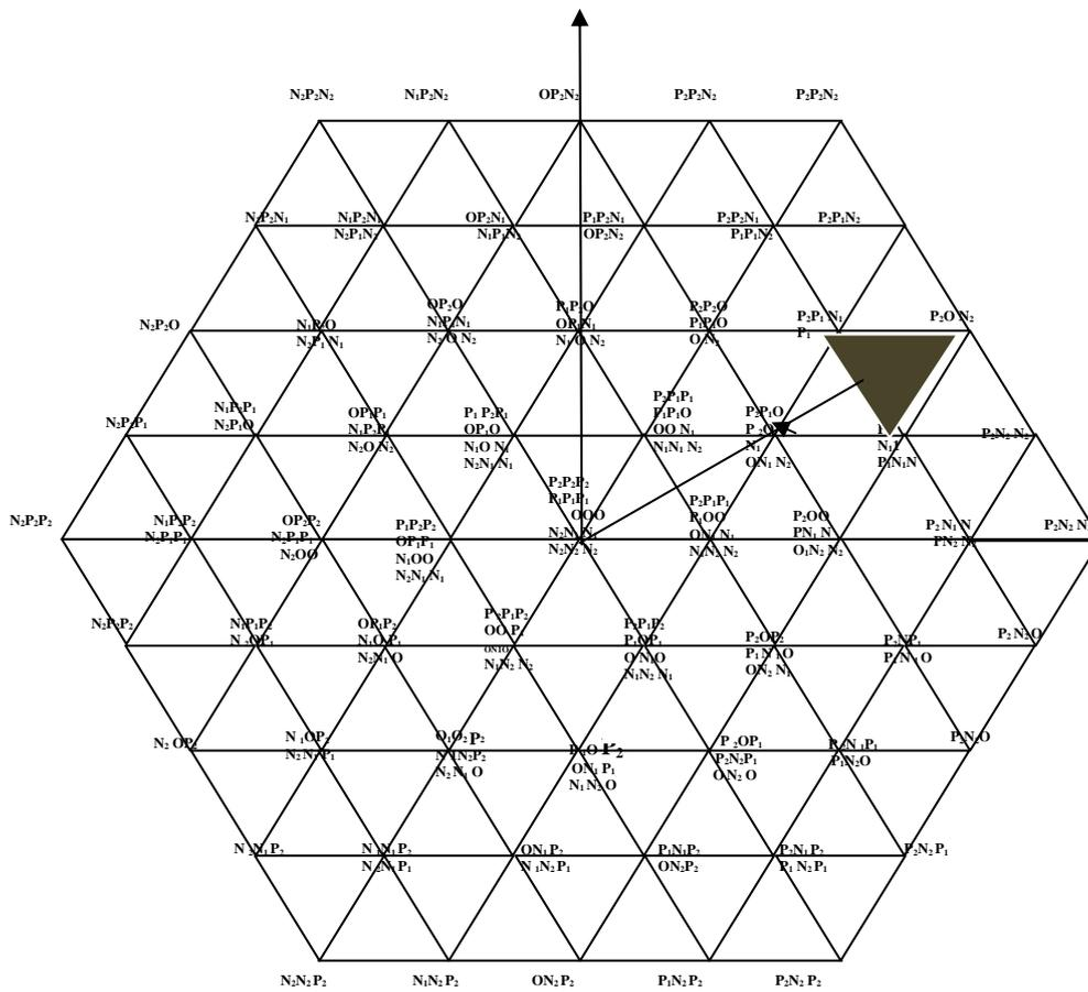
Figure 3. Space Vector diagram of Five-level inverter
