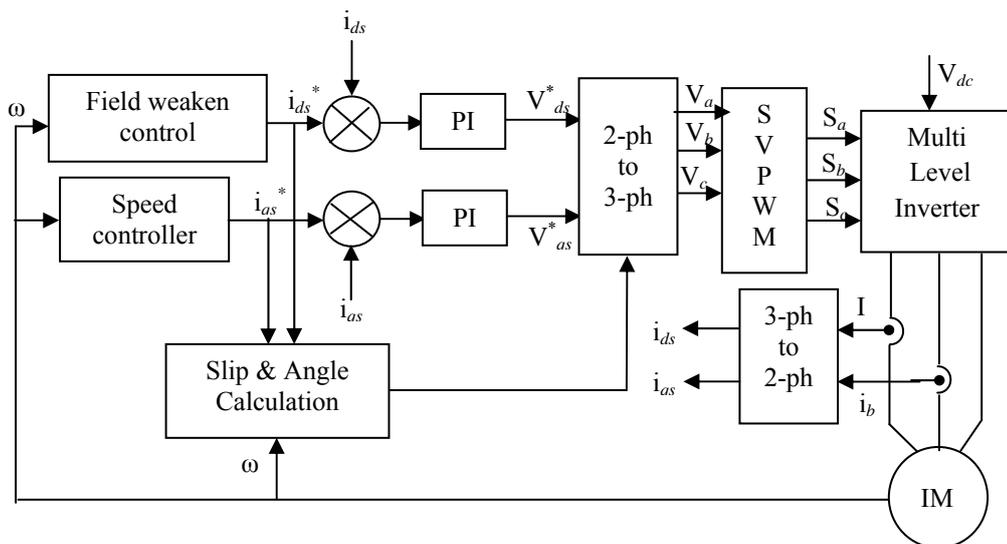
Figure 4. Block diagram of proposed Multi level inverter fed IFO based induction motor drive
