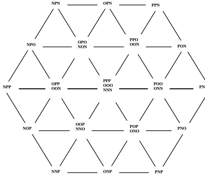
Figure 2. Space vectors of a three level inverter
