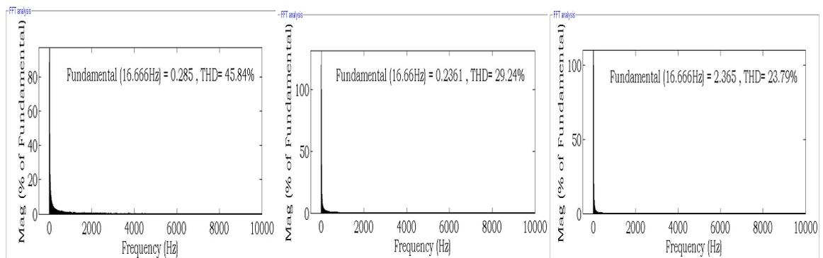
Figure 9. Harmonic spectra of line current of Two-level, Three-level and Five-Level inverter fed vector controlled induction motor drive respectively
