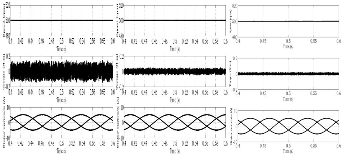
Figure 6. Steady state performance of Two-level, Three-level and Five-Level inverter fed vector controlled induction motor drive respectively
