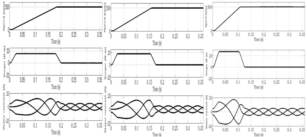
Figure 5. Starting transients of Two-level, Three-level and Five-Level inverter fed vector controlled induction motor drive respectively
