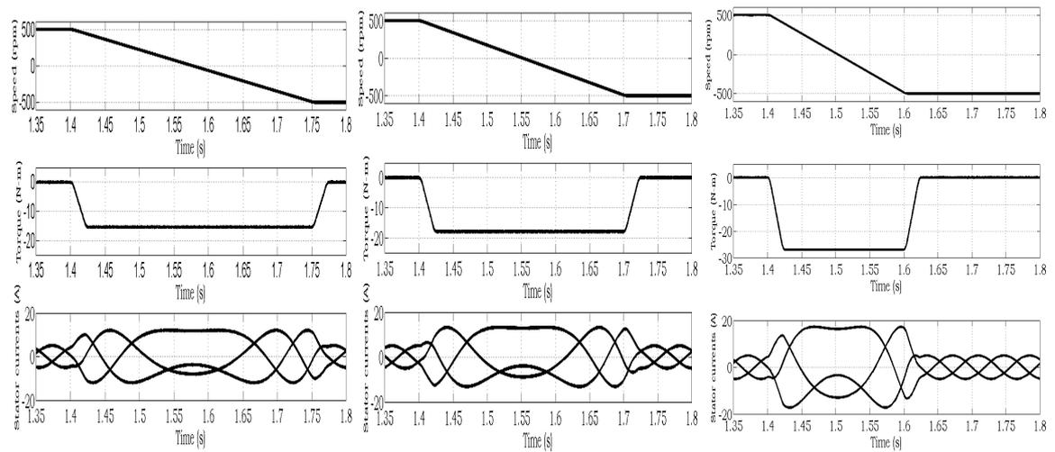
Figure 8. Performance during speed reversal operation (Speed is changed from (+500 rpm to -500 rpm) of Two-level, Three-level and Five- Level inverter fed vector controlled induction motor drive respectively
